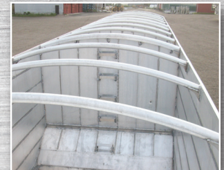
Standard Arched Top Cross Members & Vented Divider Walls
