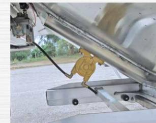
Lower hopper vibrators for fast, clean discharge
