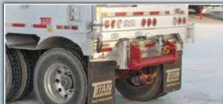
Aluminum offset push bumper with steel vertical push blocks, narrow HD tube with centre ring style pull cable.
