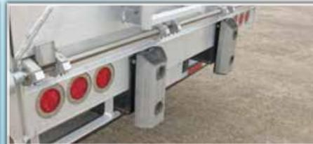
Steel flush mount with underride and stainless steel clad rubber blocks.
