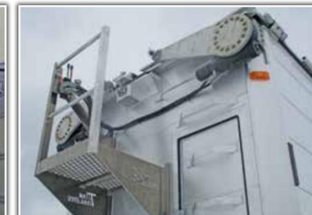
The Versitex split flip roofs are hydraulically operated using front mount slew drive gear boxes. Roofs are hinged at the sidewall using greasable heavy duty hinges. This is an excellent alternative to tarps & mesh roofs for open top trailers in terms of durability. They are comprised of a lightweight aluminum frame and Versitex composite sheet.
