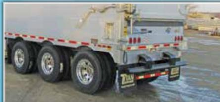
Steel offset push bumper, wide, with underride, pull cable ready.
