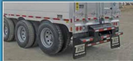
Steel offset push bumper, wide with underride. Full width steel shedder pan with tow hooks.
