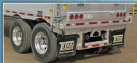
Narrow aluminum flush mount, rubber tipper bumper with T-blocks and D-ring style tow hooks.
