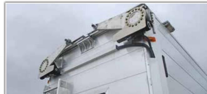
Mesh split flip roofs are hydraulically operated using front mount slew drive gear boxes. The mesh is a light weight roof option for containing the load.
