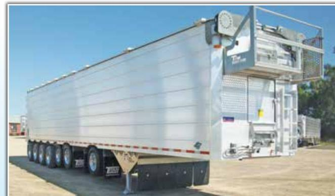
The compactor flip roofs are hydraulically operated using front mount slew drive gear boxes. Roofs are hinged at the sidewall using greasable heavy duty hinges. This allows the trailer to operate as an open or closed top trailer, providing versatility.
