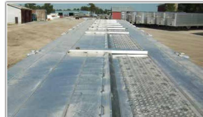
With this flip roof the trailer can be compact or top loaded. This allows the trailer to backhaul, and carry materials other than waste.
