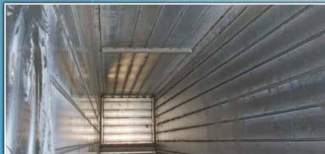
Closed top trailers feature a two-section roof. Front half consists of a lighter extruded panel profile. The rear half consists of a heavier extruded panel profile.
