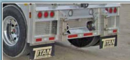
Aluminum offset bumper with filler plates and stainless steel cover with grippers and D-ring style tow hooks.
