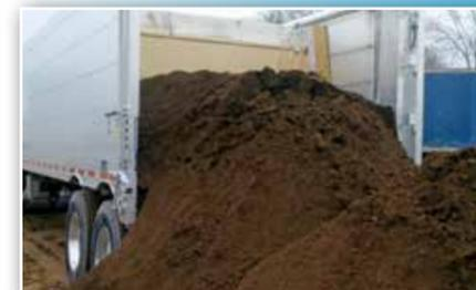
Walking floor trailer specifically designed for hauling various aggregate materials.
