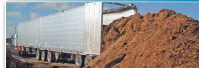
B-Train configuration, lead and pup slides together to allow material to walk from lead thru pup. Can be used on tipping platform as well.
