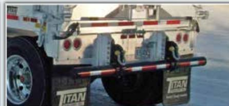
Aluminum offset push bumper with steel vertical blocks, tow shackles, full width bumper tube.
