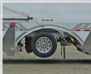
High Lift Titan ParaMAX Steer Suspension
