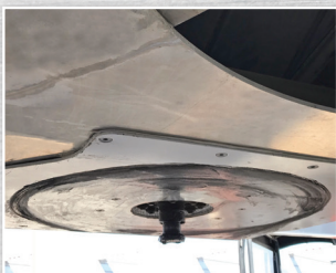
Aluminum Coupler Assembly with Bolt In Kingpin
