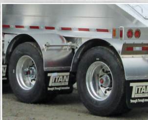
Smooth Fenders with High Clearance Pipe Brackets
