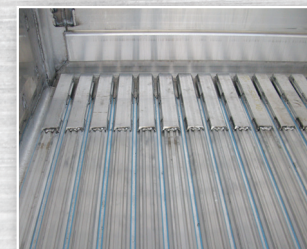
Triple Ridge 18 Slat Floor with 2' Wear Strips at Rear
