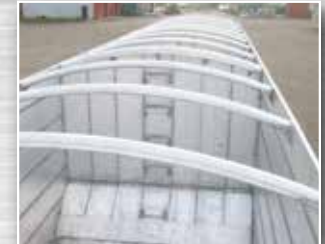
Arched Top Cross, Integrated Latch Plate & Vented Divider Walls
