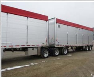
Steel Lead Chassis Aluminum Pup Chassis
