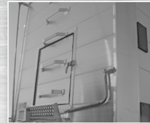
Front Access Door with Flip Down Step with Optional Rung Style Steps
