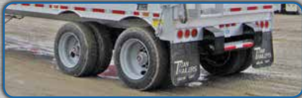
Narrow steel push pull with dirt shedders with 2 hooks incorporated into bumper.
