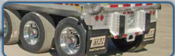
Steel vertical blocks bolted to bumper with tow shackle option for pulling, bolted to aluminum uprights.
