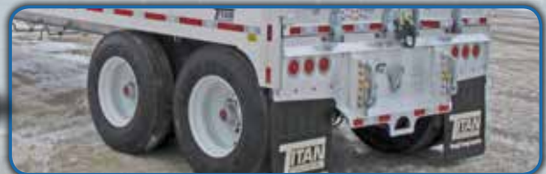
Tow shackles, with aluminum or steel vertical blocks bolted to aluminum uprights.
