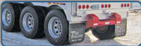
Steel pusher to accommodate centre ring style pull cable.
