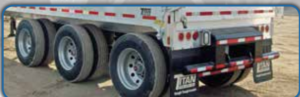
Wide, steel, offset, push with underride, tow hooks incorporated into bumper and with full width steel shedder pan on top portion
