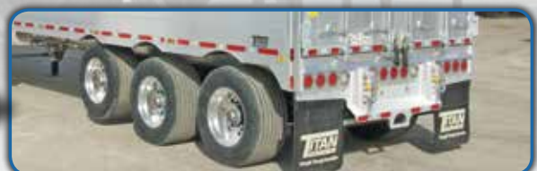
Aluminum, offset, push with underride, aluminum vertical blocks bolted to bumper and tow shackles.
