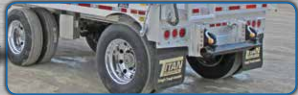
Steel pusher assembly with narrow tube, tube push bar and push bar grip plates, c/w tow shackles, steel assembly bolted in place to aluminum profiles.
