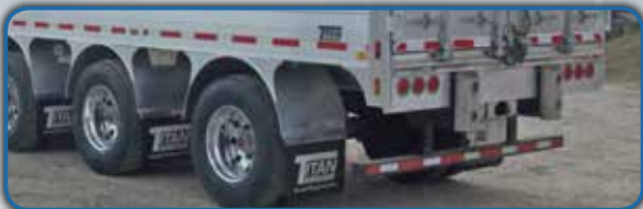
Steel, flush underride, stainless clad rubber bumper blocks.
