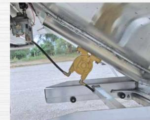
Lower hopper vibrators for fast, clean discharge
