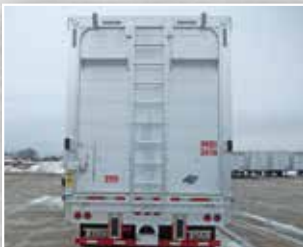
Rear Access Ladder
