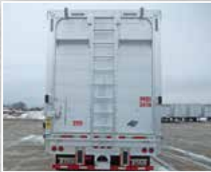
Rear Access Ladder
