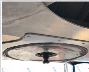
Aluminum Coupler Assembly with Bolt In Kingpin
