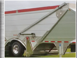
Air operated, Spring Assisted Front to Back Tarp System
