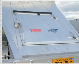
Rear Enclosure with Access to Air Tanks and Valving
