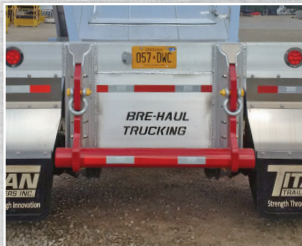
Aluminum Push Bumper with Steel Inserts, C/W Tow Shackles
