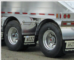
Smooth Fenders with High Clearance Pipe Brackets
