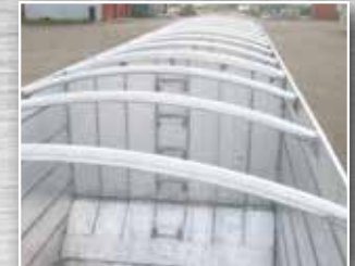
Arched Top Cross Members & Vented Divider Walls
