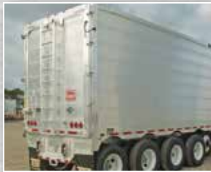
Back Ladder Centre of Rear Door
