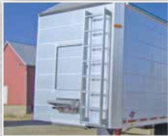
Front Ladder Drivers Side
