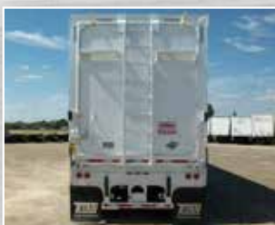
Rear Access Ladder
