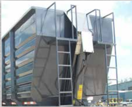
Front Catwalk/External Hoist
