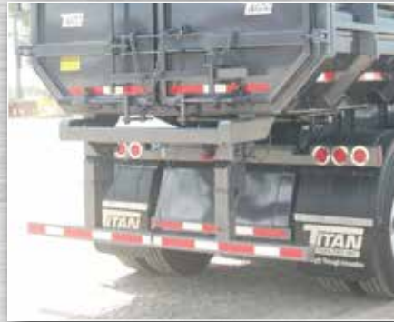
Crank Up Underride Bumper for Clearance During Dumping
