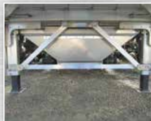
Jost All Aluminium Landing Gear
