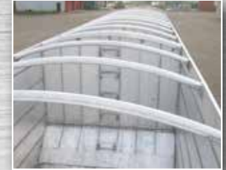
Arched Top Cross Members & Vented Divider Walls
